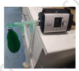
p) The Lumis 150 has now been modified. Oxygen can be supplied through the 6mm oxygen stem (4) port. The machine can be operated as usual using the desired ventilation mode and settings.
