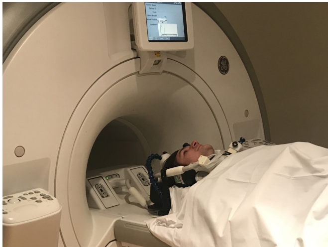
Figure 1 Coil setup, healthy volunteer demonstrating positioning of the 6CH carotid coil placed at the anterior side of the neck and secured with tape, the head is immobilised by the coil placement.
