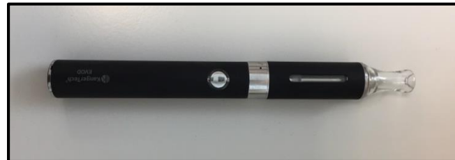
Figure E1.b Picture of Kanger e-cig used for production of ECVC/nfECVC.
