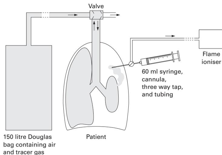
Figure 1 Diagrammatic representation of apparatus used to detect tracer gas (as previously described).<sup>4</sup>
