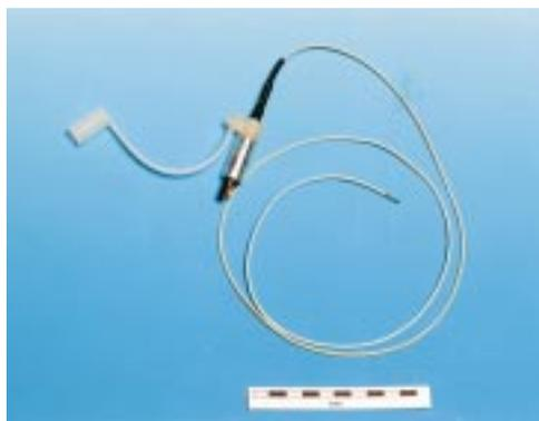
Figure 1 The micromanometer tipped pulmonary artery catheter. The external luer fitting allows injection of air for calibration. The stainless steel tip houses the transducer.
