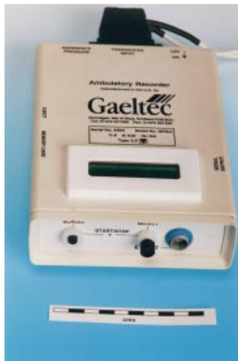
Figure 2 The ambulatory recorder. This weighs 650 g and is worn over the shoulder in a carrying case by the patient throughout the period of recording. During a recording the liquid crystal display on top of the box reads real time and percentage of memory occupied. The event button on the front of the recorder is pressed by the patient at the beginning and end of an activity or postural change, simultaneously with a calibration.
