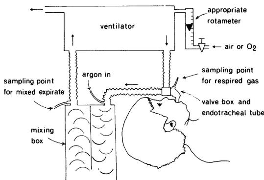
Fig 1 *Diagram of the breathing circuit.*
