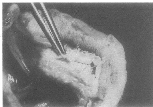
Fig 2 Exploded view of commissural-annular junction showing fracture of commissural stent.
