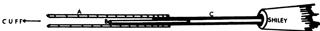
FIG. 1. 2.5 cm (ID 0.6 mm) polyethylene tubing (B) interposed between pilot tube to cuff (A) and pilot tube to clamp (C).
